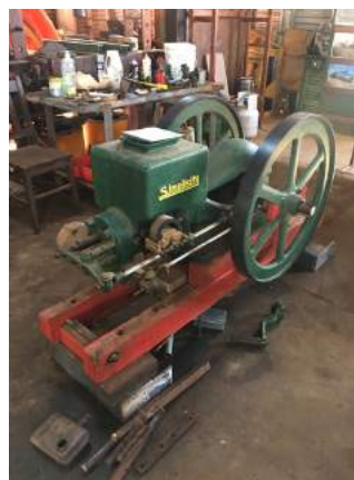
Simplicity engine out of Chaff Cutter which is also being restored.
