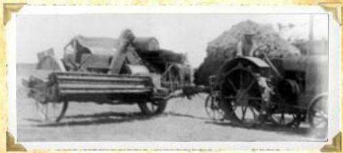
The photo, from the mid 1920's, (from a glass negative) shows a Taylor Header pulled by a McCormick Deering 15-30 tractor with solid steel wheels. (ouch). Pneumatic tires (soft ride) became available from 1933.
